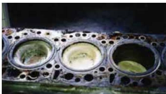
Figure 10: Picture of an Engine Damaged by Silicon
